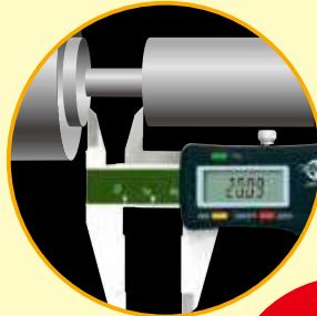
Measurement on edge face (measurement with flat-head)
